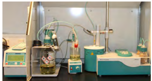
Figure 19: Equipment used for the indirect Karl Fisher method
