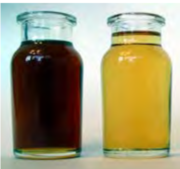
Figure 12: Degraded hydraulic oil compared to new oil Source: C.C.JENSEN A/S
